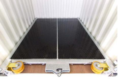
It is often difficult to reliably store and secure large systems or bulky items for transport when using standard containers. For this purpose, CHS Spezialcontainer has developed an extendable support frame. Goods weighing up to 10 tonnes can be placed and secured on the frame while it is outside of the container. The frame is then pushed back into the container and locked in place for transport. This saves time and makes loading and unloading easier.
