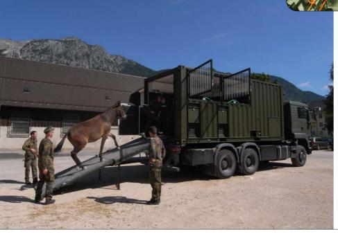
For the German Armed Forces, we developed a 20' container for transporting up to four adult riding and pack animals as well as the corresponding equipment. The pack animals can be transported safely to their destination with this container. Water tanks, troughs and temperature and video monitoring are integrated in the stable area. The ISO container animal transport also has a tack room with a pull-out staircase and its own independent heater. An awning provides protection from the weather.
