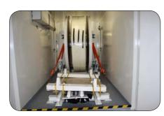
These containers accommodate a system for laying plastic pipes for pipe rehabilitation. The system consists of two mobile 20' High Cube Double Door containers that can be joined together and are able to be deployed at any location in the world. For this purpose, the containers were equipped with various doors, thermal insulation, a partition wall with an integrated pipe lead-through and a variety of foundations to accommodate the technical components of the system.
